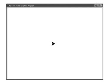
The default turtle shape is an arrowhead. (The size of the turtle shape was enlarged from its default size for clarity.) A turtle's shape can be set to basic geometric shapes, or even made from a provided image file.
