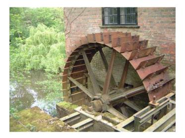
Consequently, unlike Ferris wheels that have their centers above the ground, the center of the water wheel would be placed at ground level, so the lower half of the wheel would be immersed in the stream.
